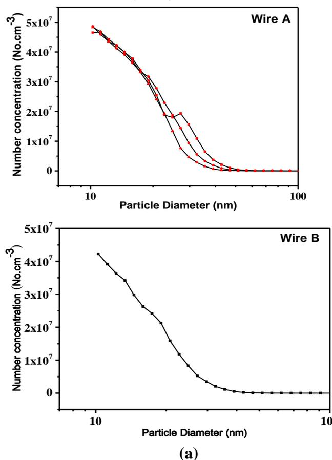
**Fig. 5: Aerosol size distribution from generator for (a) Wire A, (b) Wire B**
