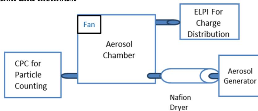
Fig.1. Experimental Set up
