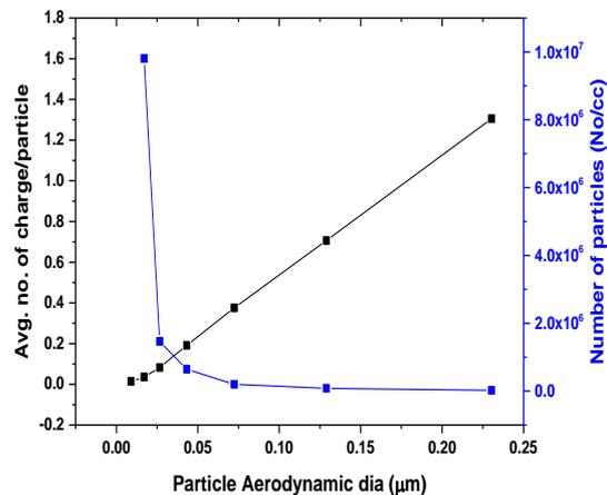
Fig.4. Particle charge and size distribution for particles generated from HWG
