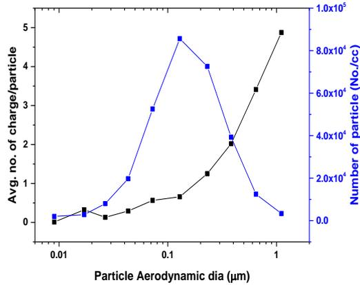
Fig.2 Particle charge and size distribution for particles generated from Nebulization of 10% NaCl solution
