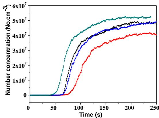
**Fig. 3: Aerosol number concentration at generator 1.0 L min<sup>-1</sup> carrier flow and applied voltage of 7 V**
