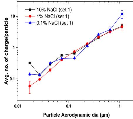
Fig.3 Particle charge distribution for particles generated from Nebulization of 10%, 1% and 0.1% NaCl solution
