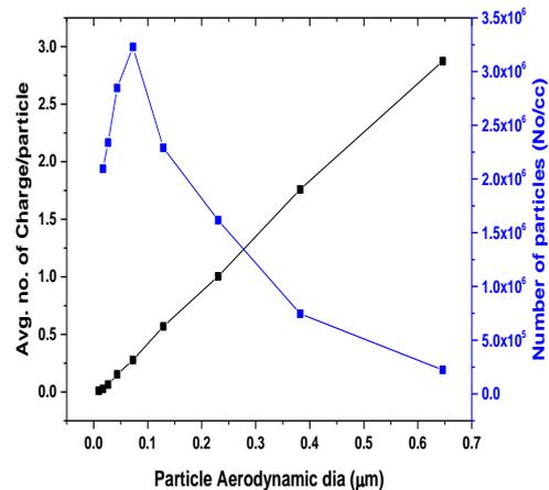
Fig.5. Particle charge and size distribution for particles generated from Combustion of Incense stick
