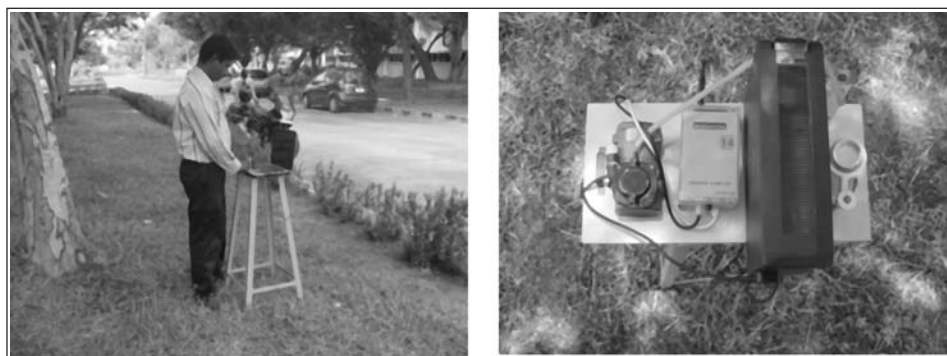
Figure 3. Photograph of the control node and the sampler system
