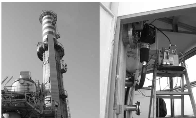
Figure 1: Chimney of the thermal waste combustion plant in Bozen and set up with the sampling probe and Wide Range Aerosol Spectrometer.
